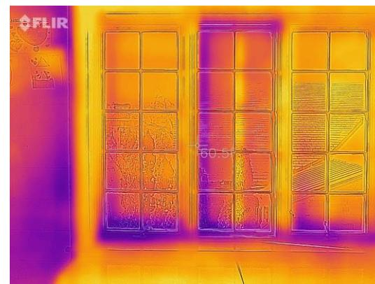
BE-23 -- Infrared photo of the 1990s windows show better thermal performance with some need to replace weatherstripping at edges.
