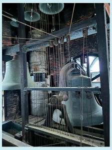
Amazingly, all of the bells, chimes, and controller was installed in the 1920s and still work today (except for that clock paper tape gizmo). The damaged coupling was replaced with a metal and plastic spider coupling, which cost about \$20. It took under an hour to replace.
